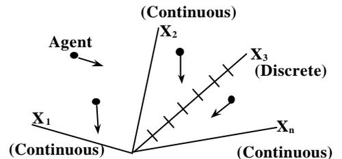
Fig. 2 Concept of expanded PSO for MINLP.
