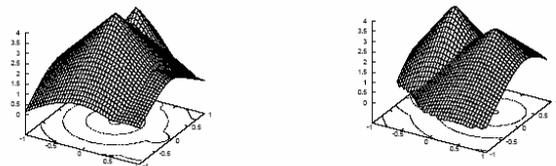
Three peak multimodal environment, before (above left) and after (above right) movement of optima. Note that the small peak to the right of the figure becomes hidden and that the highest point switches optimum (Parrott and Li, 2006).
